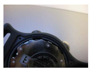
**Step 8.** Securely tighten the four screws so the case back is flush with the watch.
