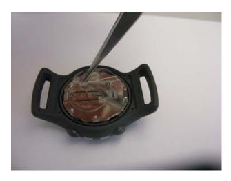
**Step 4**. Unlatch the clip covering the CR 2032 battery
