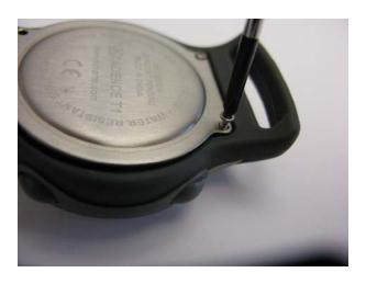
**Step 5**. Remove and replace the CR 2032 battery with a new lithium battery
