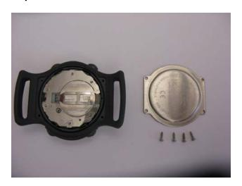
**Step 1**. Remove the four screws from the stainless steel case back of the watch with a Jewelers screwdriver
