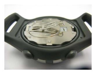
**Step 6**. Check the clips next to each button to make sure they are still aligned properly
