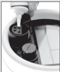
1. Apply Nyogel grease to each of the sockets. Be careful not to overfill, a small amount is needed.
