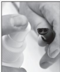
1. Use alcohol to clean the inside of the connector sockets.
