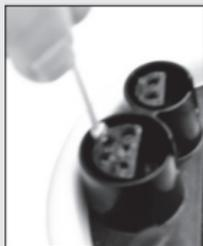
3. Using foam swab, apply Nyogel to the entire outside of both rubber connectors, not the plastic.
