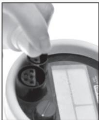
1. Use alcohol to clean the inside of all the connector sockets
