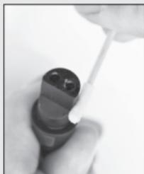
3. Using foam swab, apply Nyogel to the entire outside of rubber connector.
