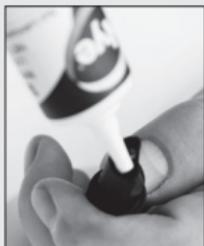
1. Apply Nyogel grease to both sockets. Be careful not to overfill, a small amount is needed.
