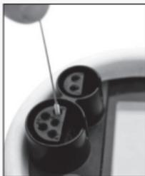
2. Insert supplied metal brush into each socket several times to loosen and clean debris
