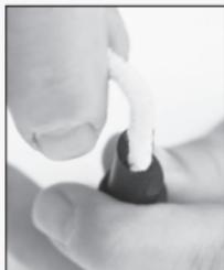
3. Next use a pipe cleaner to remove any excess alcohol and debris.
