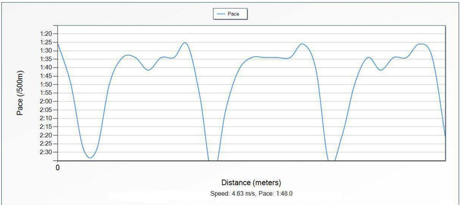
We can see the “camel backs” in set-up A, while B is slightly smoother and maintained a higher overall speed, being over 5% faster than A.
