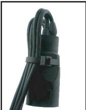
1) Locate the 4-pin rubber plug (R4) which plugs into the front panel of the Cox-Box. The receptacle is in the shell and connects the wiring harness to the Cox-Box. Cut the zip tie that secures the wires to the plug. Be careful not to nick the wires!
