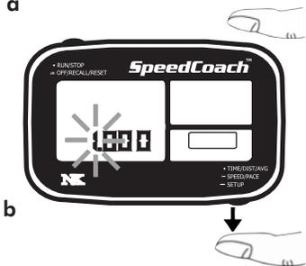
Press the bottom button to change this number. Hold bottom button for 1 second to move between digits (c). Repeat hold and press to move through and change all appropriate digits (d). Hold to exit.
